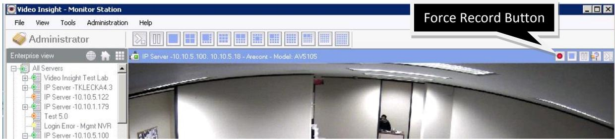
Selecting this option does not permanently change the camera's recording type. Clicking the Force Record button forces the camera to record and when complete the camera will resume its normal recording setting.
