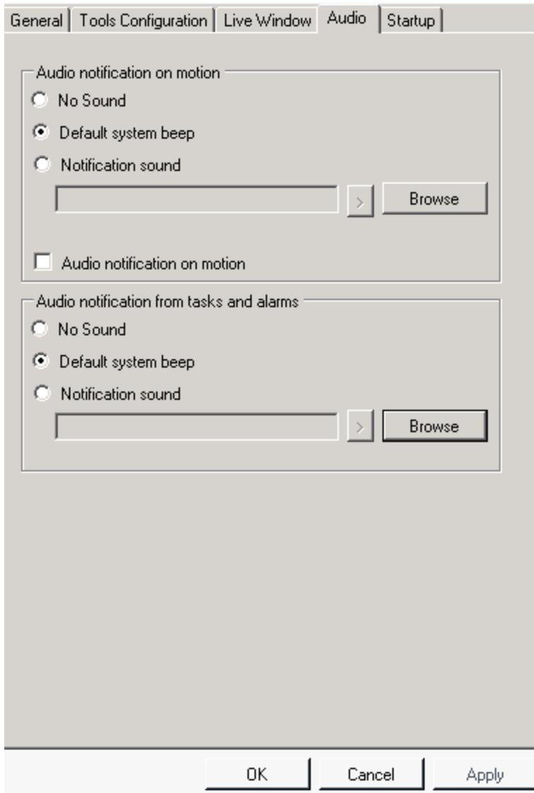
**Audio notification on motion:** You can select this option to give the user the ability to specify if there will be audio notification when motion is detected on a camera. You have the option of no sound, default system beep or you can load your own notification sound by browsing to a .WAV file.
